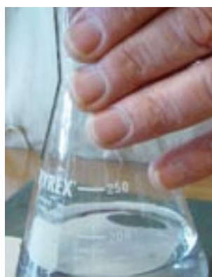
Figure 5 The endpoint of the titration is reached when just enough thiosulfate is added to react with all the iodine present and the solution becomes colourless.
