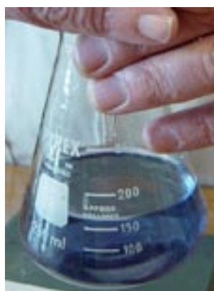
Figure 4 As more thiosulfate is added and we near the titration endpoint, the blue-black colour from the starch-iodine complex fades.
