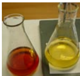
Figure 2 Titration of the iodine formed. The left flask shows the brown-coloured solution resulting from the formation of iodine. The right flask shows how the brown colour fades to pale yellow as the iodine is titrated with thiosulfate (this is the stage at which starch solution should be added).
