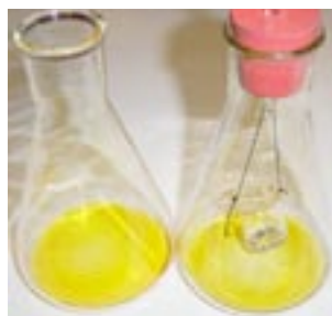
Figure 1 Experimental setup for oxidation of ethanol. Conical flask contains yellow acid dichromate solution and is sealed with rubber stopper. Small beaker containing beverage sample is suspended above from hook in rubber stopper.
