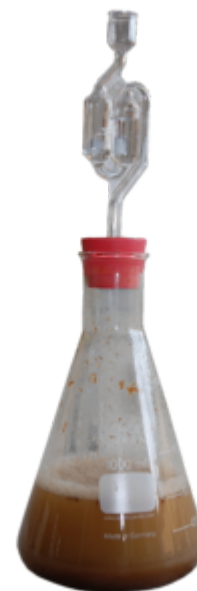
A laboratory vessel being used for the fermentation of straw.
