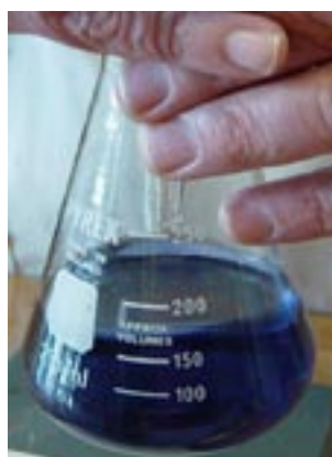
Figure 3 Upon addition of starch the solution takes on a blue-black colour due to the formation of a starch-iodine complex.
